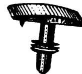
73-3906 Replaces: 3981457 CLIP-ROOF HEADER WEATHERSTRIP Side Front Door Window Glass Weatherstrip Hole: 1/4", Head: 1/4" X 3/4", P.R.: 5/16" Blazer '71 - '72 General Purpose UNIT PACKAGE 100
