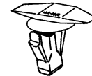
99-8114 Replaces: N806289-S, N806340-S RETAINER- WEATHERSTRIP Plastic Hole: M4.8, Head: 5 x 15MM, P.R.: .8 - 1.95MM Ford F150 Pick Ups '97/ UNIT PACKAGE 100
